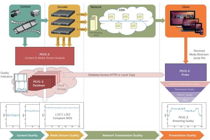
**Example OTT Network and PEVQ-S Building Blocks**: PEVQ-S is split into a hybrid architecture, consisting of two major blocks: the **Content & Media Stream Analysis** (left, applied at the server side), and the **Client Probe** (right) analyzing the Transmission and Presentation Quality and processing the final MOS score.
