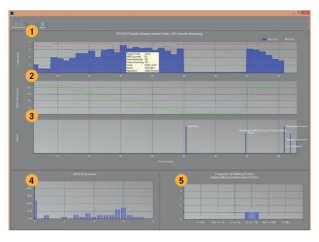
CVQ MOS indicates the actual limitation in quality due to lower connectivity and adaptive bit rate switching and characterizes the transmission quality of the network.
